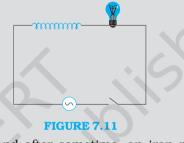
The switch is closed and after sometime, an iron rod is inserted into the interior of the inductor. The glow of the light bulb (a) increases; (b) decreases; (c) is unchanged, as the iron rod is inserted. Give your answer with reasons.
