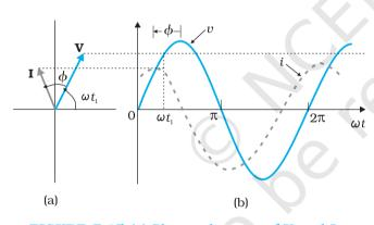
FIGURE 7.15 (a) Phasor diagram of V and I.
