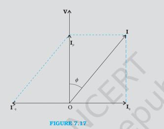
the applied voltage **V** and **I**<sub>q</sub> perpendicular to the applied voltage. **I**<sub>q</sub> as you have learnt in Section 7.7, is called the wattless component since corresponding to this component of current, there is no power loss. **I**<sub>p</sub> is known as the power component because it is in phase with the voltage and corresponds to power loss in the circuit.
