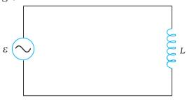
**FIGURE 7.5** An ac source connected to an inductor.
