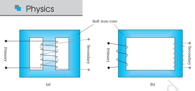
**FIGURE 7.20** Two arrangements for winding of primary and secondary coil in a transformer: (a) two coils on top of each other, (b) two coils on separate limbs of the core.
