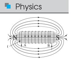
**0-1** Current *i* through the coil entering at A increase from zero to a maximum value. Flux lines are set up i.e., the core gets magnetised. With the polarity shown voltage and current are both positive. So their product *p* is positive. ENERGY IS ABSORBED FROM THE SOURCE.
