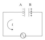
**2-3** As *i* continues to flow from A to B, the capacitor is charged to reversed polarity i.e., the plate B acquires positive and A acquires negative charge. Both the current and the voltage are negative. Their product p is positive. The capacitor ABSORBS ENERGY during this 1/4 cycle.
