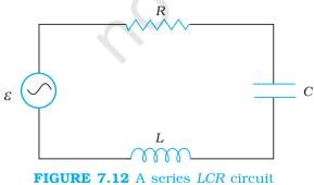
connected to an ac source.
