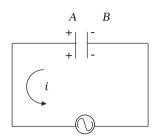
**1-2** The current *i* reverses its direction. The accumulated charge is depleted i.e., the capacitor is discharged during this quarter cycle. The voltage gets reduced but is still positive. The current is negative. Their product, the power is negative.
