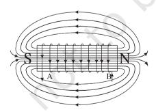
**2-3** Current *i* becomes negative i.e., it enters at B and comes out of A. Since the direction of current has changed, the polarity of the magnet changes. The current and voltage are both negative. So their product p is positive. ENERGY IS ABSORBED.
