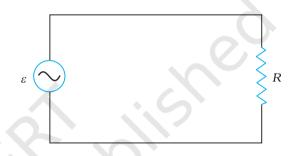
FIGURE 7.1 AC voltage applied to a resistor.
