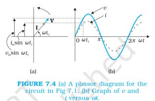
voltage and current phasors on vertical axis, i.e.,  $v_m \sin \omega t$  and  $i_m \sin \omega t$ , respectively represent the value of voltage and current at that instant. As they rotate with frequency  $\omega$ , curves in Fig. 7.4(b) are generated.
