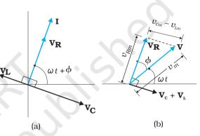
**FIGURE 7.13** (a) Relation between the phasors  $\mathbf{V}_{L}$ ,  $\mathbf{V}_{R}$ ,  $\mathbf{V}_{C}$ , and *I*, (b) Relation between the phasors  $\mathbf{V}_{L}$ ,  $\mathbf{V}_{R}$ , and  $(\mathbf{V}_{L} + \mathbf{V}_{C})$  for the circuit in Fig. 7.11.
