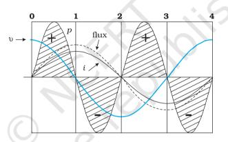
One complete cycle of voltage/current. Note that the current lags the voltage.
