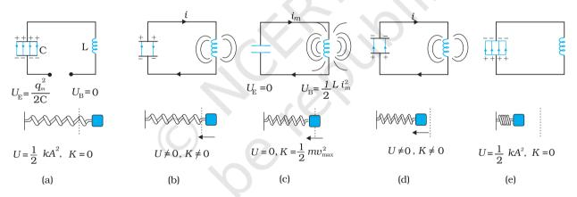
**FIGURE 7.19** The oscillations in an *LC* circuit are analogous to the oscillation of a block at the end of a spring. The figure depicts one-half of a cycle.
