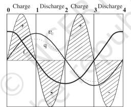
One complete cycle of voltage/current. Note that the current leads the voltage.
