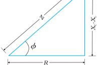
Since phasor **I** is always parallel to phasor  $\mathbf{V}_{\mathbf{R}}$ , the phase angle  $\phi$  is the angle between  $\mathbf{V}_{\mathbf{R}}$  and **V** and can be determined from Fig. 7.14:
