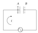
**0-1** The current *i* flows as shown and from the maximum at 0, reaches a zero value at 1. The plate A is charged to positive polarity while negative charge q builds up in B reaching a maximum at 1 until the current becomes zero. The voltage  $v_c = q/C$  is in phase with q and reaches maximum value at 1. Current and voltage are both positive. So  $p = v_c i$  is positive. ENERGY IS ABSORBED FROM THE SOURCE DURING THIS QUARTER CYCLE AS THE CAPACITOR IS CHARGED.
