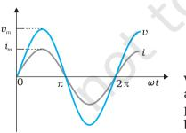
**FIGURE 7.2** In a pure resistor, the voltage and current are in phase. The minima, zero and maxima occur at the same respective times.
