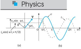
**FIGURE 7.9** (a) A Phasor diagram for the circuit in Fig. 7.8. (b) Graph of v and i versus  $\omega t$ .
